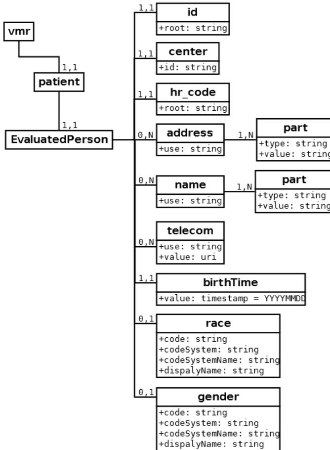
Figure 5.3: Diagram of the XML tags for the patient's demographics.
