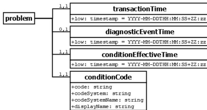
Figure 5.7: Diagram of the XML *problem* tag.
