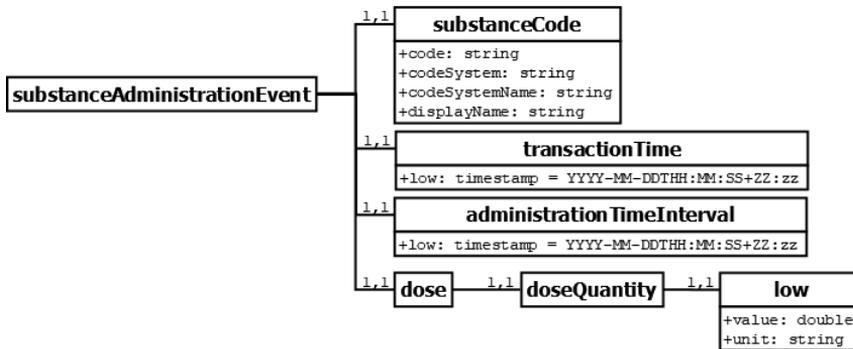
Figure 5.10: Diagram of the XML *substanceAdministrationEvent* tag.
