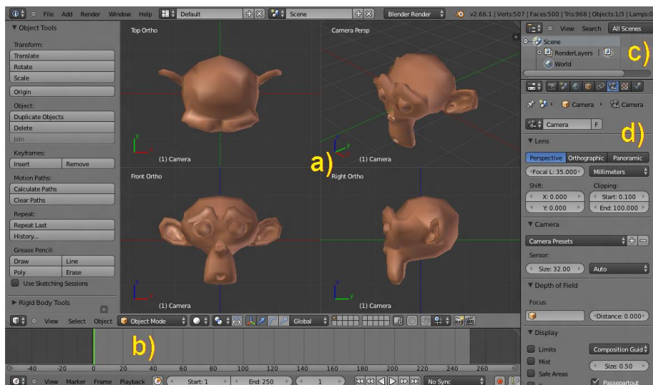
Figure 60: Blender's main GUI. In its default configuration it is made up of 4 windows: the 3D view (a), the Timeline (b), the Outliner (c) and the Properties (d)
