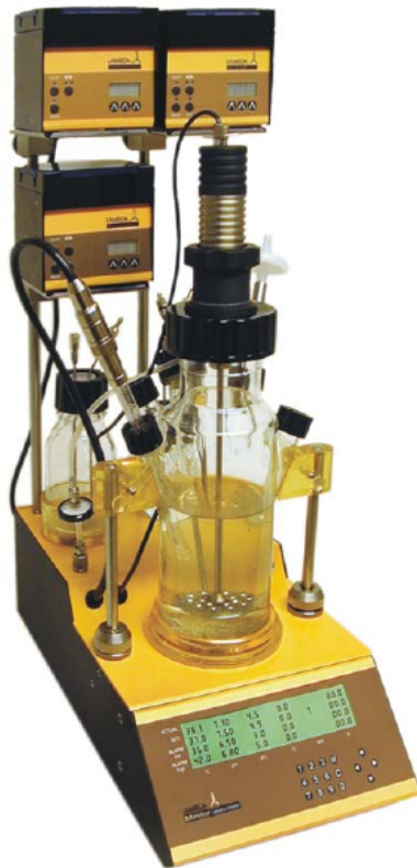
Figure 2.2: The LAMBDA MINIFOR fermenter-bioreactor. Photograph of the fermenter-bioreactor used in this work to maintain liquid cultures at a constant OD_{600} .
